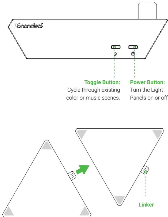
To connect the panels together, insert a linker into the linker port on the reverse of the Light Panels. Ensure that the metal contacts are aligned, and gently connect the panels together.
