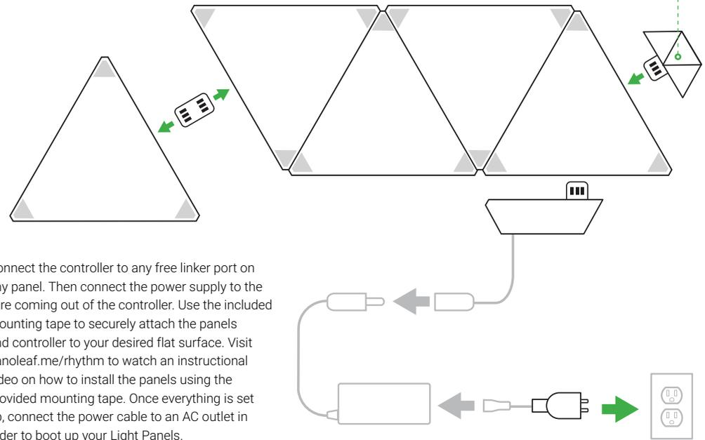
Connect the controller to any free linker port on any panel. Then connect the power supply to the wire coming out of the controller. Use the included mounting tape to securely attach the panels and controller to your desired flat surface. Visit [nanoleaf.me/rhythm](https://nanoleaf.me/rhythm) to watch an instructional video on how to install the panels using the provided mounting tape. Once everything is set up, connect the power cable to an AC outlet in order to boot up your Light Panels.
