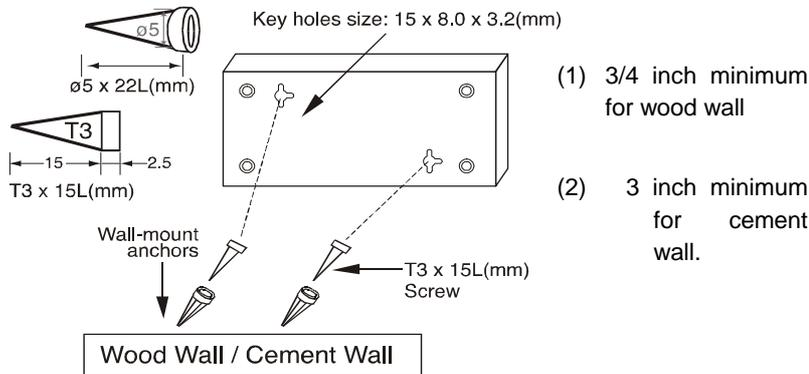
Figure 2-1. Mounting the Switch to a Wall
