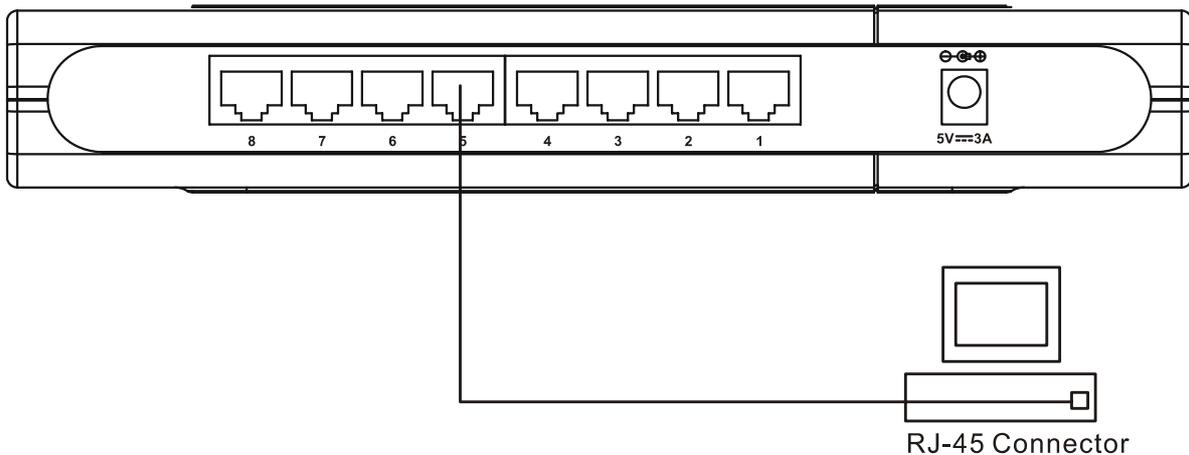
**Figure 3-1. Switch connected to an end node**
