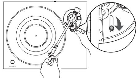
4. While still lightly holding the headshell, turn the counterweight to adjust the tonearm's balance.
