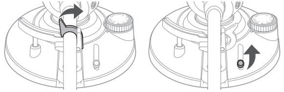
3. Place the tonearm over the rubber mat. Hold the headshell and lower the tonearm lift control lever completely.
