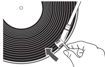
5. Lower the tonearm by moving the tonearm lift control lever to the DOWN position. The tonearm descends slowly onto the record and play begins.
