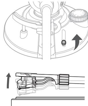
4. Position the tonearm over the desired location (groove) on the record.
