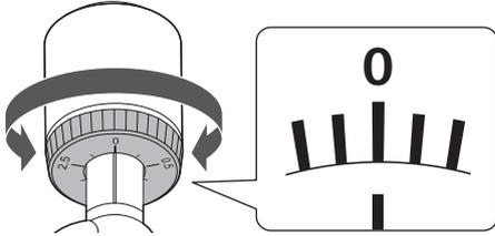
2. Turn the counterweight and the tracking force gauge ring together counterclockwise (to the left) until the centerline value matches the recommended tracking force value for the cartridge you are using.
