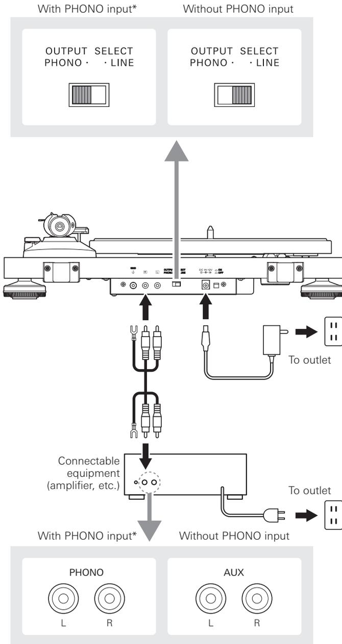
\* Depending on the equipment you are connecting, a ground (earth) terminal may exist near the phono input jack. If this is the case, connect to it using the ground line from the RCA audio cable. This may help prevent a low humming noise that might otherwise be heard during playback.
