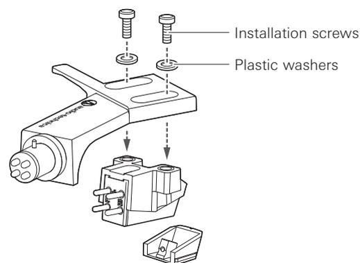
6. Using a commercially sold, non-metallic slotted screwdriver, tighten the screws in both places, and then adjust the overhang.
