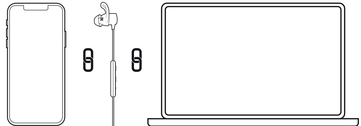
Your Tarah can remember up to eight paired Bluetooth® devices and can be actively connected two devices at a time.
