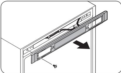
1. Remove the screw and pull out the **control cover**.
