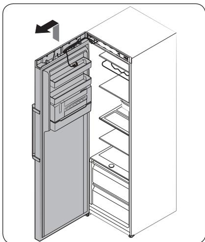
4. When the **top hinge** is removed, lift up to remove the freezer door. Keep the door in a safe place.
