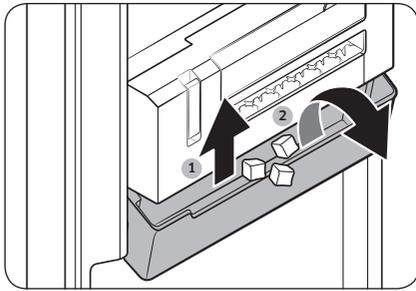
3. To dispense ice, slightly lift up the **ice bucket** and tilt to the front.
