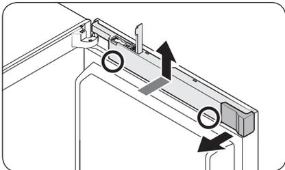
1. Open the **dongle cover**, and remove the **space cover**.
