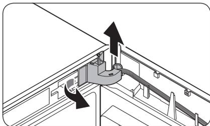
2. Pull out the left side of the **hinge cover** to remove, and then slightly lift up the bottom to pull out.
