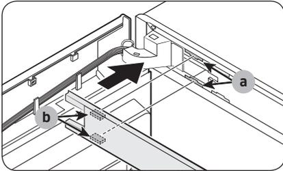
9. Insert the **top frame cover** with the **part (a)** fitting in the **part (b)** diagonally.
