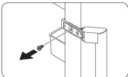
2. Remove each screw on the upper and lower side of the handle.
