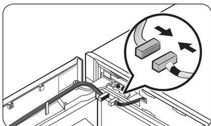
7. Connect the connectors from the freezer door and the main unit. Then, fix the wires on the inner hook of the optional hinge cover (L).
