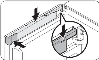
11. Insert the **space cover (L)** into the original position, and then close the **dongle cover**.
