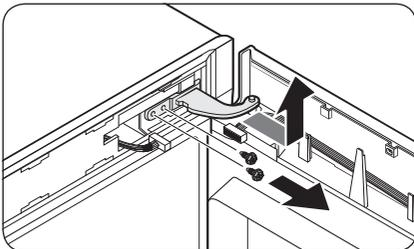
1. Remove the **top frame cover** from the right side first. Then, pull out to the front.
