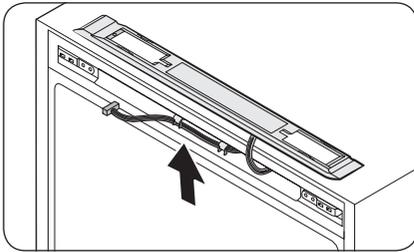
2. Move the connectors and wires to the opposite side. Insert the control cover, and then tighten the screws on the opposite side.
