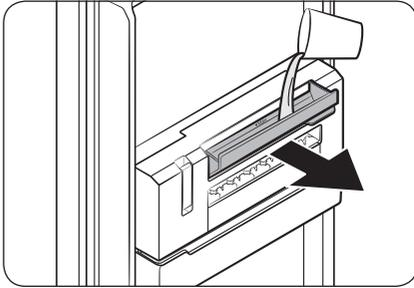
1. Pull up the handle of the **water bin (01)** to open, and then fill the bin with water up to the max line. Gently close the bin so that water does not drop or leak.
