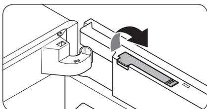
1. Open the freezer door, and pull up to open the dongle cover at the top of the door.
