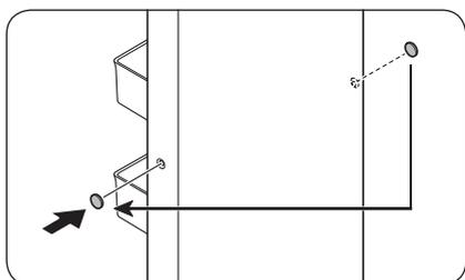
3. Use a flat-head screwdriver to remove the **handle screw caps** (x2). Then, insert the **handle screw caps** in the opposite side.
