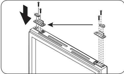
1. From the freezer door, remove the **auto closer lever** by loosening the screws on the lever and the screws in the opposite side.
