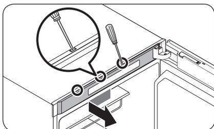
1. Use a flat-head screwdriver to insert in the holes one after another on the top of the door to remove the **top frame cover**.
