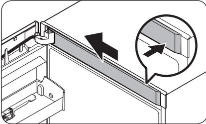
10. Insert the **wire cover** through the opened **dongle cover**. Turn the cover by 90 degrees to the front, and then push down to fit in.
