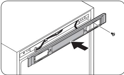
3. Remove the **shaft** from the **top hinge**. Then, reassemble the **shaft** as shown.
