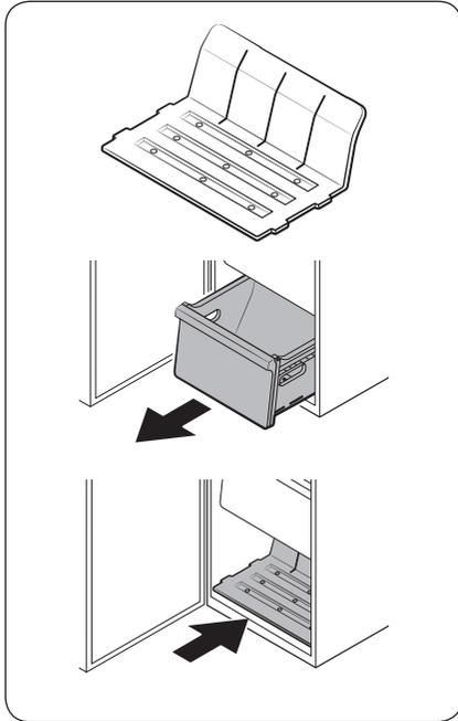
If you need more storage space, remove the top shelf cover and all 4 drawers and insert the provided shelf (see the figure) in the inner bottom of the main unit. Then, remove the Slim Ice Maker.
