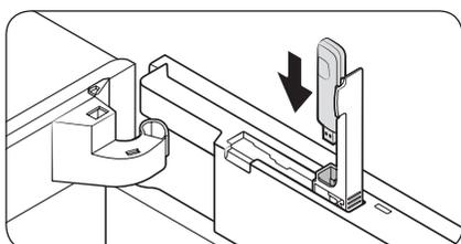
2. Insert the Smart Home Dongle into the dongle port in the correct direction.
