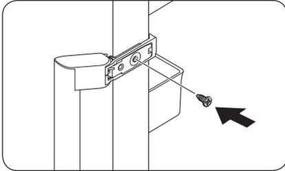
1. Insert the handle in the opposite side, and then tighten the screw.
