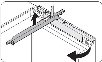
3. Turn the **wire cover** to the front by 90 degrees, and then push up to remove.
