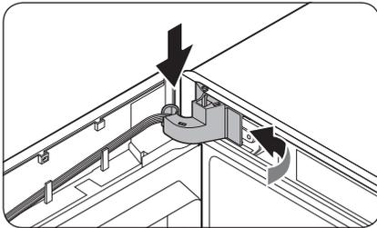
8. Insert the **hinge cover** in the **top hinge** with the right side first. Then, press the bottom of the cover to fit.
