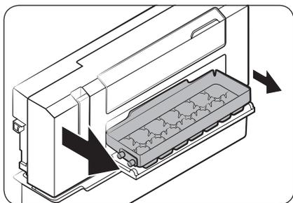
2. Slightly pull out the left side of the **ice template**, and then pull out the other side to remove.
