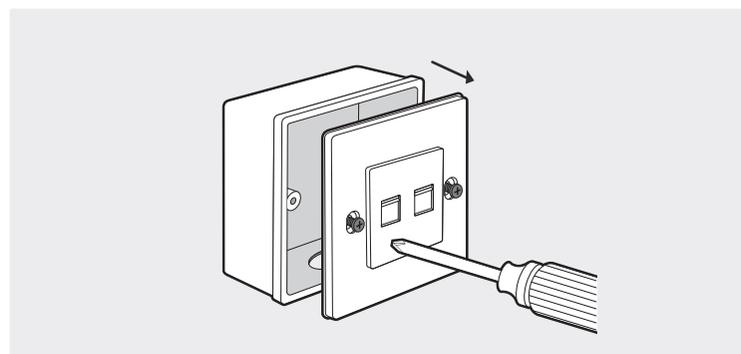
2. Detach the faceplate of the EAP with a screwdriver.
