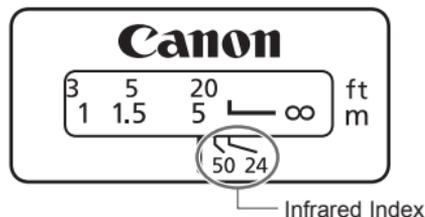
The infrared index corrects the focus setting when using monochrome infrared film. Focus on the subject manually, then adjust the distance scale indicated by the distance index by moving the focusing ring to the corresponding infrared index mark before shooting.
