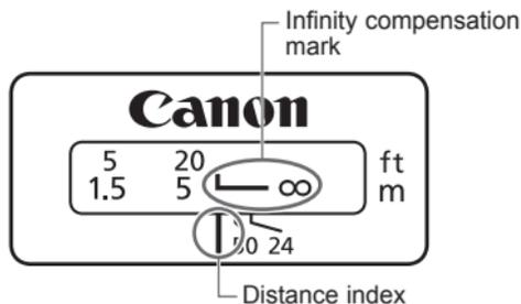
To compensate for shifting of the infinity focus point that results from changes in temperature, there is a margin at the infinity ( $\infty$ ) position. The infinity position at normal temperature is the point at which the vertical line of the distance scale L mark is aligned with the distance index.
