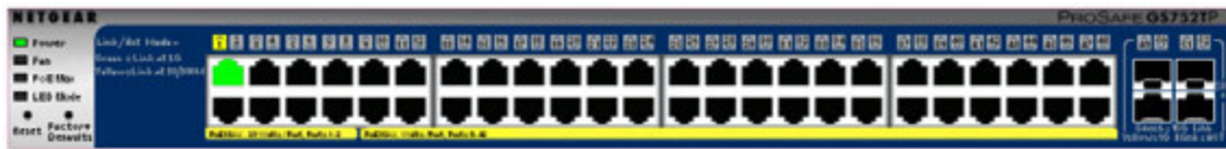
Figure 2. Ports and LEDs on the Switching Devices
