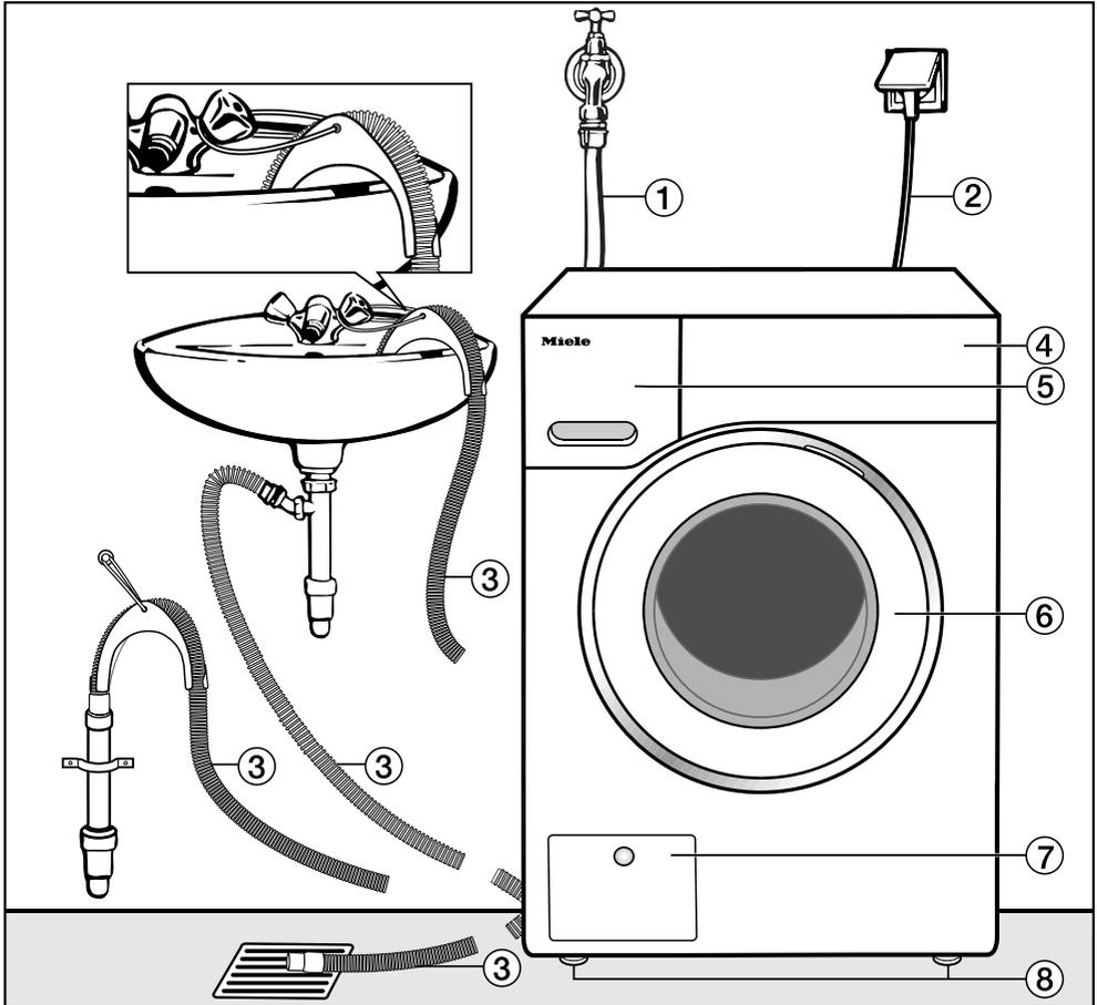
① Inlet hose (tested to withstand pressure of at least 7,000 kPa)
