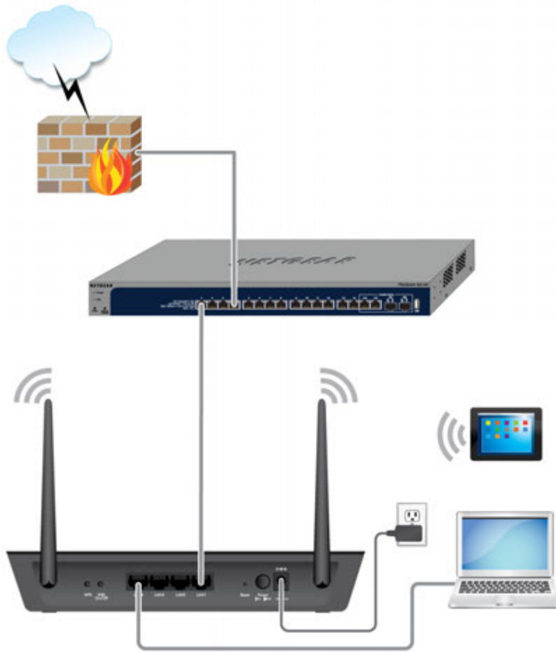
Figure 7. Connect the access point with a static IP address to a network
