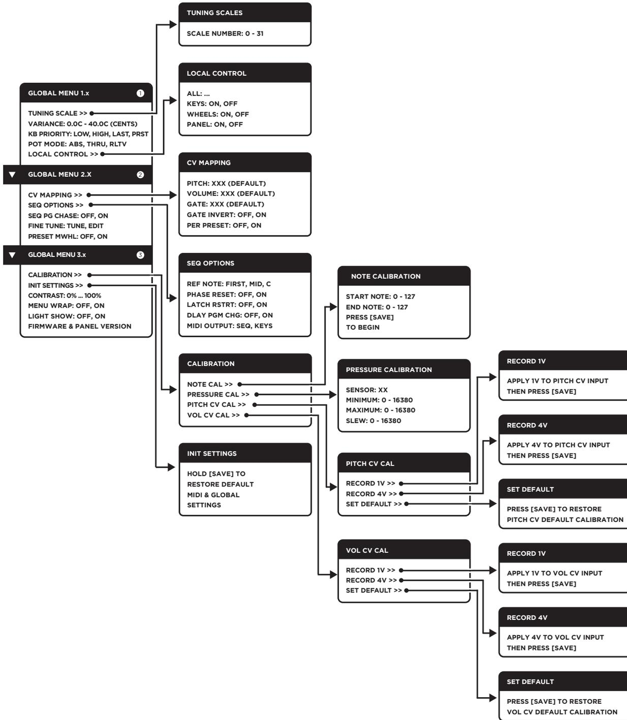
Pressing the **GLOBAL** button takes you to the **GLOBAL MENU**, which contains parameters that affect all presets. When the **GLOBAL** button is illuminated the top right of the LED display will indicate which page you are on, followed by a decimal point, and then which parameter line you have selected. Use the ▼ ▲ buttons to choose a parameter for editing, and the **FINE TUNE** knob to scroll through a selected parameter's available options.
